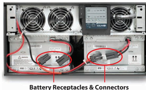
Figure 26: Disconnecting the battery packs (front view)
